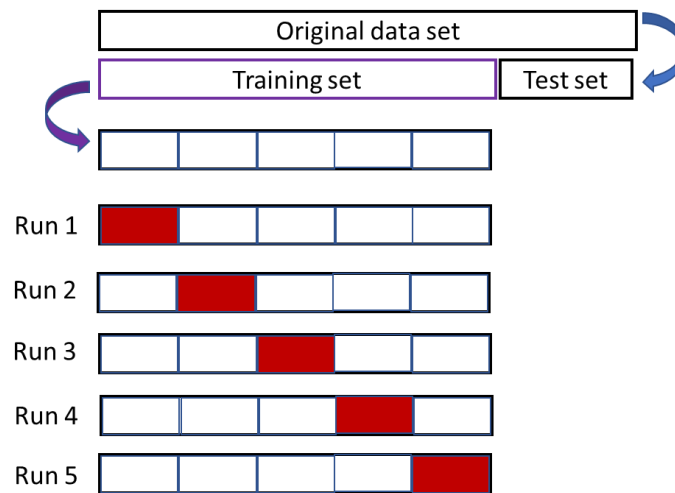
Fig.6.9 K-fold cross-validation ( K=5 ): the red box indicates the validation set for the run.
