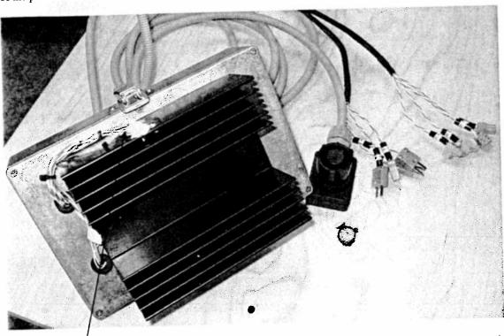
There are three extra thermocouples on the fins (T6, T7, T8) that require connection to the control console extra sockets. These are fitted with thermocouple plugs that match the sockets on the console. Note that duplex thermocouples are no longer supplied as thermocouples connect through the digital temperature indicator to the Hilton Data logger
