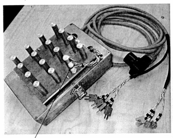
There are three extra thermocouples on the pins (T3, T4, T5) that require connection to the control console extra sockets. These are fitted with thermocouple plugs (shown above) that match the sockets on the console.
