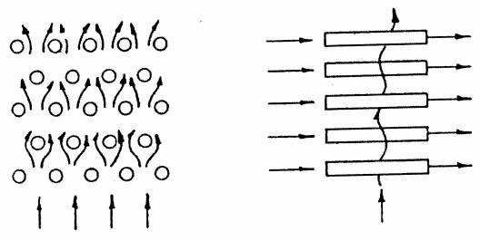
Various tube and fin layouts have been devised in order to improve the efficiency heat exchangers and thereby reduce the physical size for a given heat transfer rate. However, the objective of all of the arrangements is to promote turbulence in the fluid flowing across the extended surfaces.
