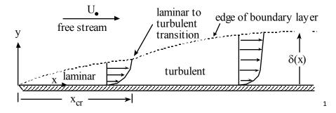
The velocity distribution in the laminar boundary layer is relatively simple in that it is governed by one relation. The boundary layer height, " $\delta$ ", occurs at the height, "y", where  $u(y) = 0.99U_{\infty}$ .
