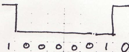
Bipolar AMI      1 = Neg or pos - alternate      0 = No line signal
