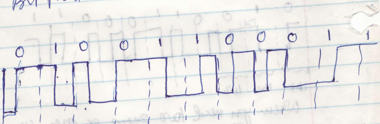
For fast ethernet, Multilevel transitions (MLT-3) is used. A change in voltage indicates 1, no change near zero. There are 5 voltage levels used.
