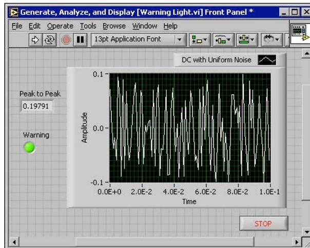
Figure 2-1 Front panel for the Warning Light VI
