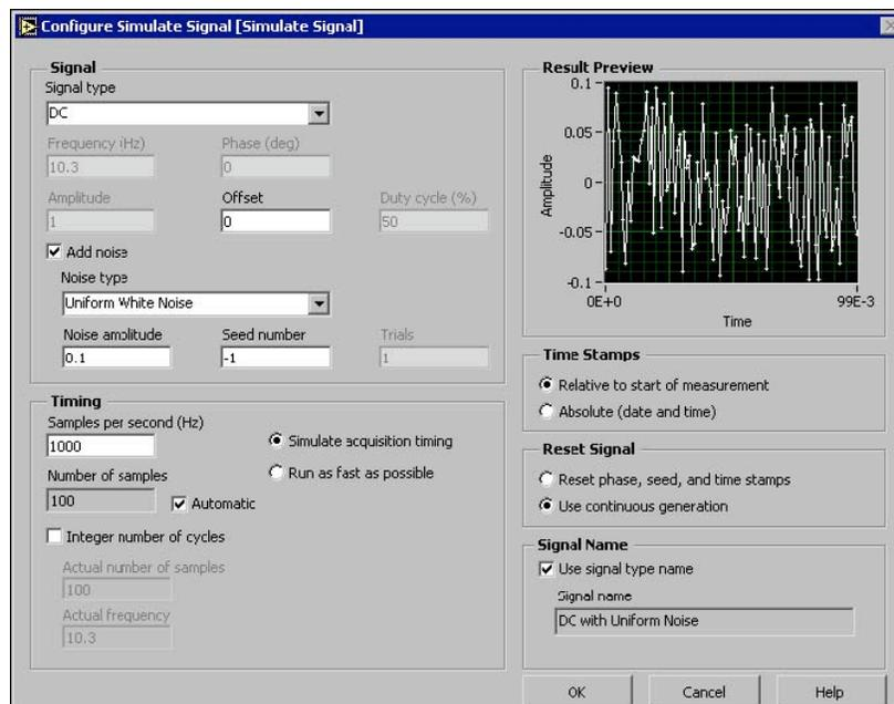
Figure 2-3 Configure Simulate Signal Dialog Box
