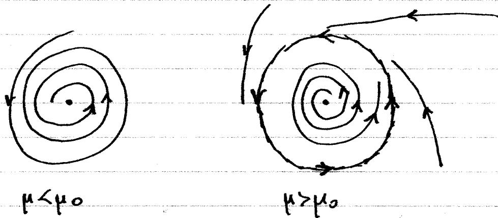
A stable spiral fixed point for  $\mu < \mu_0$  becomes an unstable spiral for  $\mu > \mu_0$  surrounded by a stable limit cycle which expands with increasing  $\mu$ .
