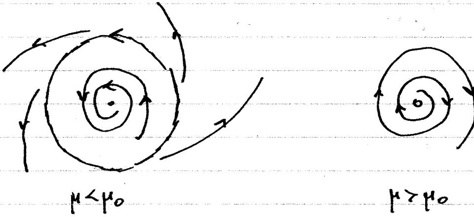
At  $\mu < \mu_0$ , a stable spiral is bounded by an unstable limit cycle. With increasing  $\mu$ , the unstable limit cycle becomes smaller.
