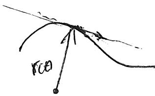
$T(t)$  tangent to trajectory follows direction of motion
