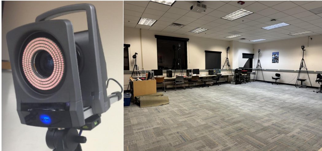
Fig. 1 Vicon camera (left), laboratory (right): Overview of the laboratory and camera arrangement used to record overground walking at 100 Hz. A single subject performed normal walking and asymmetrical load carriage (farmer's carry) trials, including postfatigue conditions following sets of body-weight squats. Marker trajectories were used to compute knee clinical angles via a modified Grood–Suntay joint coordinate system.
