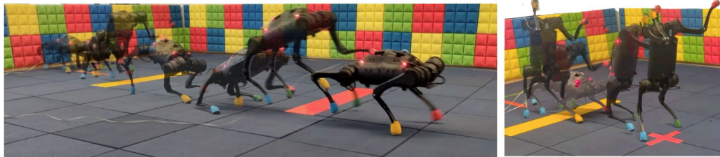
Fig. 1: Agile skills learned with our proposed method enable the A1 robot to jump repeatedly (left) and walk to a goal location on its hind legs (right).
