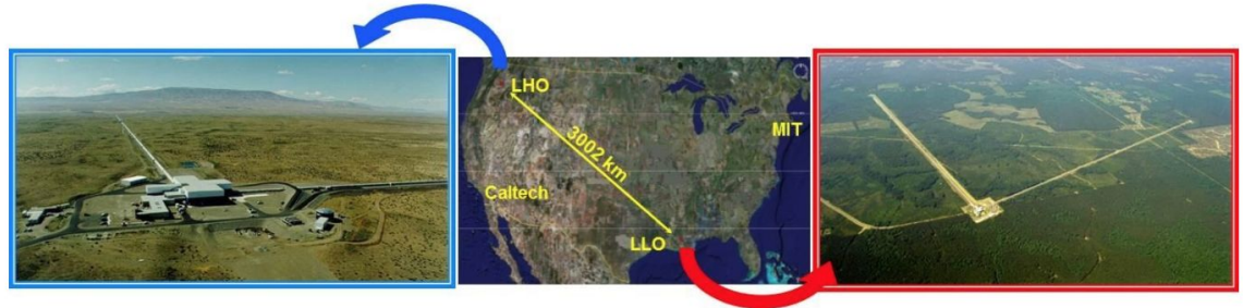
Figure 3 The two LIGO detectors at Hanford, Washington (left) and Livingston, Louisiana (right). Each L-shaped interferometer has 4 km long optical cavities.
