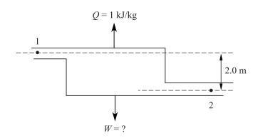
The steady flow energy equation is
