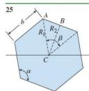
Regular polygon with n sides (Origin of axes at centroid)
