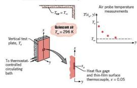
The following table provides measurements from the heat flux sensor at six *x*-locations for the specified plate–air temperature difference.
