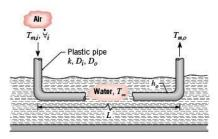
If air from the home enters the pipe at a temperature of  $T_{m,i} = 29^{\circ}\text{C}$  and a volumetric flow rate of  $V_i = 0.025 \text{ m}^3/\text{s}$ , what pipe length L is needed to provide a discharge temperature of  $T_{m,o} = 21^{\circ}\text{C?}$  What is the fan power required to move the air through this length of pipe if its inner surface is smooth?
