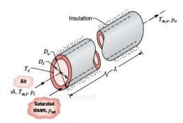
Consider conditions for which air enters a 50-mm-diameter tube at a pressure of 5 atm, a temperature of  $T_{m,i} = 17^{\circ}\text{C}$ , and a flow rate of  $\dot{m} = 0.03$  kg/s, while saturated steam at 2.455 bars condenses on the outer surface of the tube. If the length of the annulus is L = 5 m, what are the outlet temperature  $T_{m,o}$  and pressure  $p_o$  of the air? What is the mass rate at which condensate leaves the annulus?
