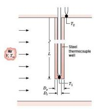
for steel,  $k = 35 \text{ W/m} \cdot \text{K}$ , and, for air,  $\rho = 0.774 \text{ kg/m}^3$ ,  $\mu = 251 \times 10^{-7} \text{ N} \cdot \text{s/m}^2$ ,  $k = 0.0373 \text{ W/m} \cdot \text{K}$ , and Pr = 0.686.
