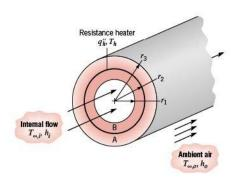
Liquid pumped through the tube is at a temperature  $T_{\infty,i}$  and provides a convection coefficient  $h_i$  at the inner surface of the composite. The outer surface is exposed to ambient air, which is at  $T_{\infty,o}$  and provides a convection coefficient of  $h_o$ . Under steady-state conditions, a uniform heat flux of  $q_h^n$  is dissipated by the heater.
