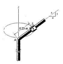
13-77. The 2-kg spool S fits loosely on the inclined rod for which the coefficient of static friction is  $\mu_s = 0.2$ . If the spool is located 0.25 m from A, determine the maximum constant speed the spool can have so that it does not slip up the rod.
