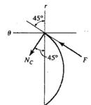
13-109. The collar, which has a weight of 3 lb, slides along the smooth rod lying in the horizontal plane and having the shape of a parabola  $r=4/(1-\cos\theta)$ , where  $\theta$  is in radians and r is in feet. If the collar's angular rate is constant and equals  $\dot{\theta}=4\,\mathrm{rad/s}$ , determine the tangential retarding force P needed to cause the motion and the normal force that the collar exerts on the rod at the instant  $\theta=90^\circ$ .
