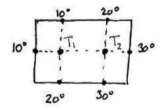
$$\begin{array}{rcrcrcrcrc} T_1 & = & \frac{10+10+T_2+20}{4} & \Rightarrow & 4T_1 & - & T_2 & = & 40 \\ T_2 & = & \frac{T_1+20+30+30}{4} & \Rightarrow & -T_1 & + & 4T_2 & = & 80 \end{array}$$
