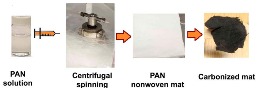
FIG. 1. Schematic of the input and output process for PAN-based carbon fiber production using the Forcespinning (FS) technique. [Color figure can be viewed at wileyonlinelibrary.com ]
