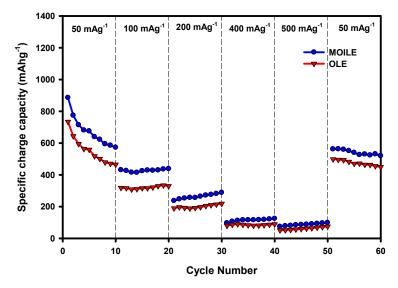
**Figure 10.** Rate performance (charge capacity vs cycle number at different current densities) of  $SnO_2/C$  composite fibers at 25 °C with two different electrolytes: OLE (1M LiPF<sub>6</sub> in EC/DMC (1:1 v/v)), and MOILE (1 M LiTFSI in 60% EMI-TFSI/ 40% EC/DMC (1:1 v/v) with 5 wt% SN).
