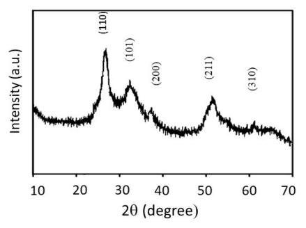
**Figure 4.** XRD pattern of the SnO<sub>2</sub>/C composite-fiber membrane prepared after calcination of PAN/SnO<sub>2</sub> precursor fibers at 700 °C.
