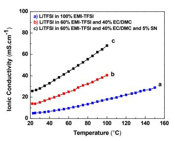
**Figure 5.** Ionic conductivity vs temperature for the ionic liquid electrolyte (ILE), mixed organic/ionic liquid electrolyte (MOILE), and MOILE with 5 wt.% SN.
