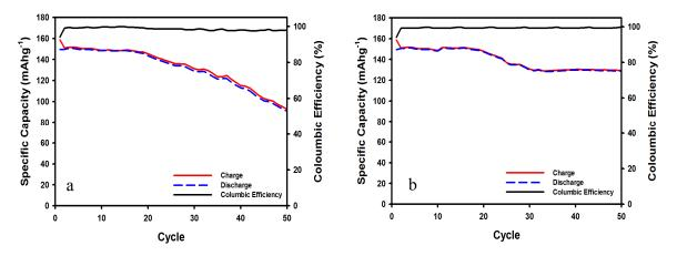
**Figure 7.** Cycling performance and coulombic efficiency of LiCoO<sub>2</sub> commercial cathode at 60 °C in (**a**) 1 M LiTFSI in 60% EMI-TFSI 40% EC/DMC (1:1 v/v) electrolyte, and (**b**) 1 M LiTFSI in 60% EMI-TFSI 40% EC/DMC (1:1 v/v) with 5 wt% SN. Current density = 100 mA g<sup>-1</sup>.
