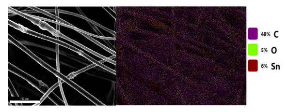
**Figure 2.** SEM image of SnO<sub>2</sub>/C composite fibers (left) and corresponding EDS mapping of the SnO<sub>2</sub>/C composite fibers (right).
