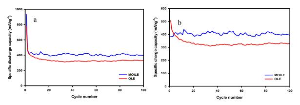
**Figure 9.** Cycling performance of a SnO<sub>2</sub>/C composite-fiber anode at 25 °C in two different electrolytes: (a) 1M LiPF<sub>6</sub> in EC/DMC (1:1 v/v) electrolyte, and (b) 1 M LiTFSI in 60% EMI-TFSI/ 40% EC/DMC (1:1 v/v) with 5 wt% SN.
