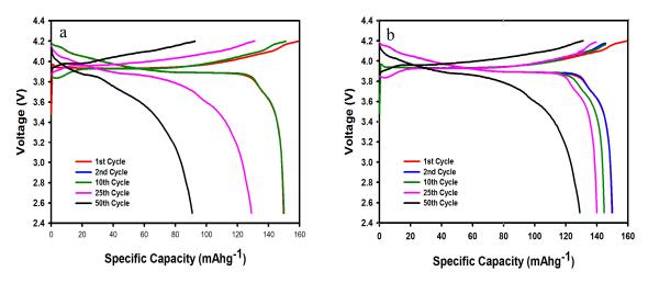
**Figure 6.** Charge/discharge profiles of a commercial LiCoO<sub>2</sub> cathode at 60 °C with MOILEs (**a**) 1 M LiTFSI 60% EMI-TFSI 40% EC/DMC EC/DMC (1:1 v/v), and (**b**) 1 M LiTFSI 60% EMI-TFSI 40% EC/DMC EC/DMC (1:1 v/v) containing 5 wt% SN. Current density = 100 mA g<sup>-1</sup>.
