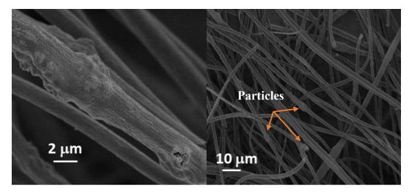
**Figure 1.** SEM images of a SnO<sub>2</sub>/C composite-fiber membrane [20], with copyright permission from the IOP Publishing.
