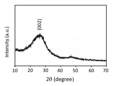
**Figure 3.** XRD pattern of the carbon-fiber membrane prepared after the carbonization of polyacrylonitrile (PAN) fibers at 700 °C.
