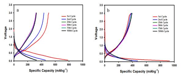
**Figure 8.** Charge/discharge profiles for a SnO<sub>2</sub>/C composite-fiber anode at 25 °C in two different electrolytes: (**a**) 1M LiPF<sub>6</sub> in EC/DMC (1:1 v/v) electrolyte, and (**b**) 1 M LiTFSI in 60% EMI-TFSI/ 40% EC/DMC (1:1 v/v) with 5 wt% SN.
